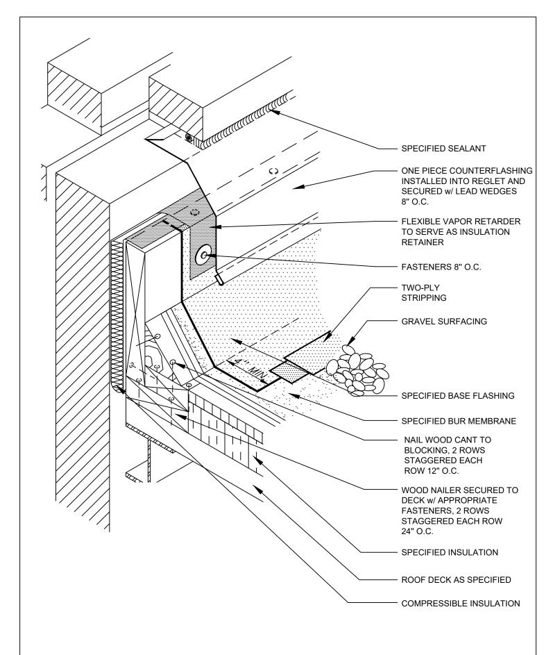
BUILT-UP ROOF HOT/COLD WALL FLASHING FOR NON-WALL-SUPPORTED DECK
