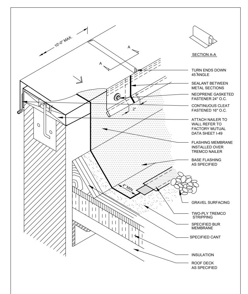
BUILT UP ROOFING HOT/COLD LIGHT METAL PARAPET CAP
